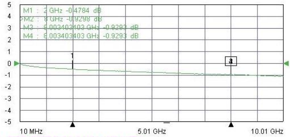
Tr4 S22 Refl SWR RefLvl: 1 U Res: 100 mU/Div
